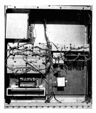
Phaselocked 10080 MHz local oscillator and 288 MHz SSB transverter. 10 MHz standard in upper left.
